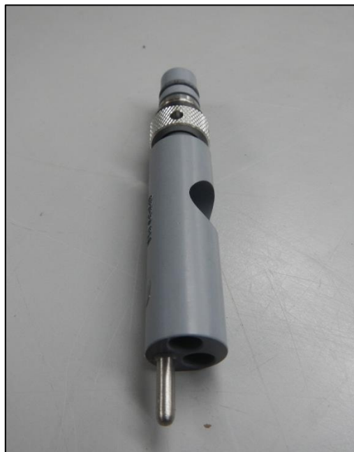
Figure 20: YSI 6560 Temperature/Conductivity Sensor
