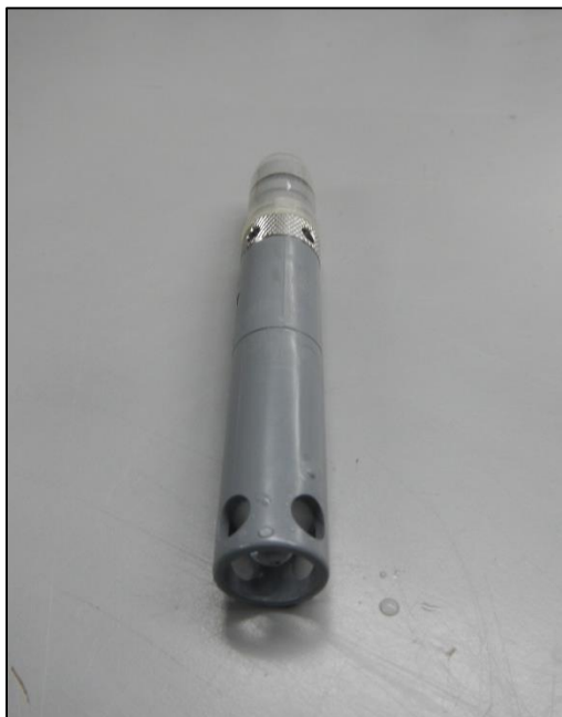
Figure 19: YSI 6561 pH Sensor
