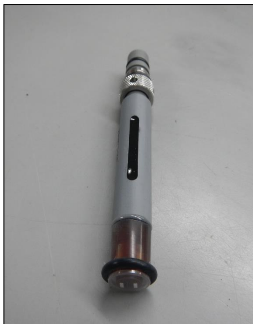
Figure 22: YSI 6562 Dissolved Oxygen Sensor
