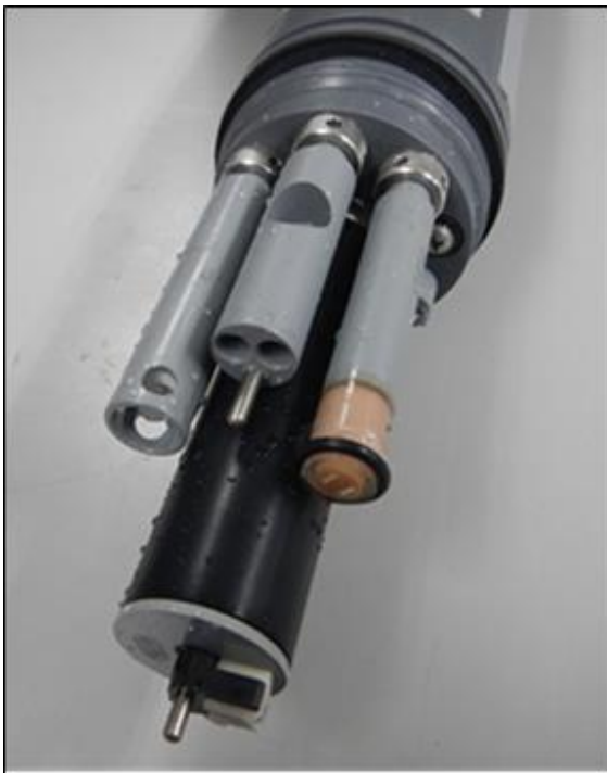
Figure 18: YSI 6820 Multi-parameter Sonde from Side (Left) and Front (Right)
