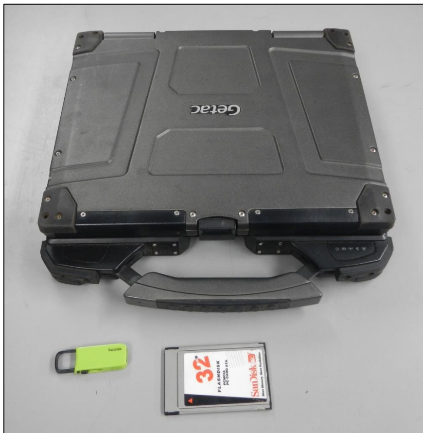
Figure 26: Field Data Transfer Equipment
