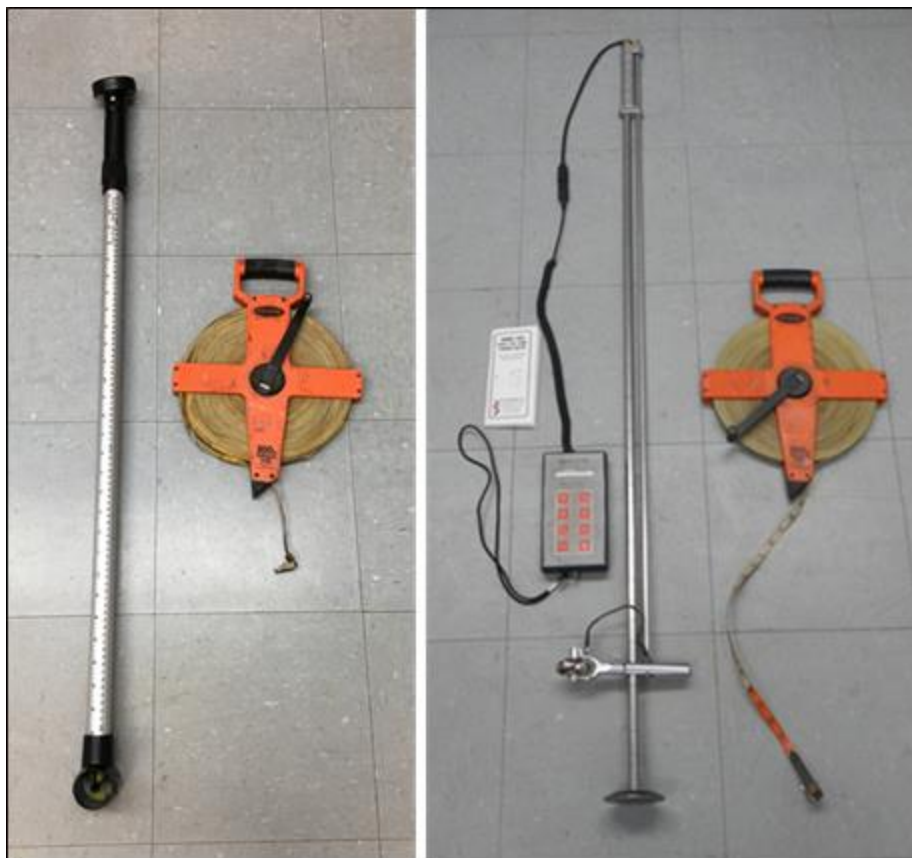
Figure 16: Flow Measurement Equipment
