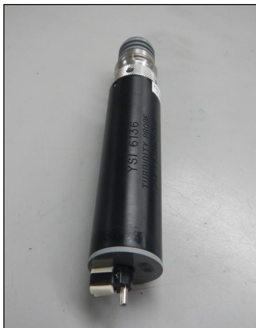
Figure 21: YSI 6136 Turbidity Sensor
